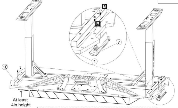
1. Place the table top on the platform at least 4in height during installation to prevent crushing and scratching the light device.
